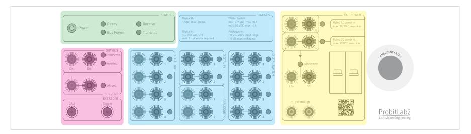
ProbitLab2's DALI bus and related measurement connections.
